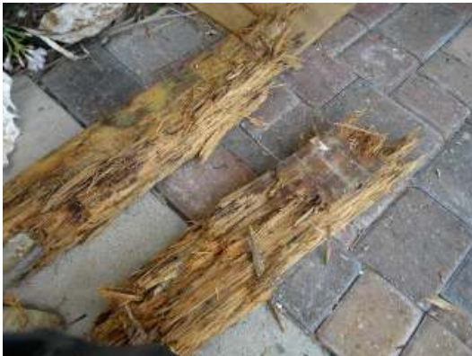
Remains of a laminated beam.
